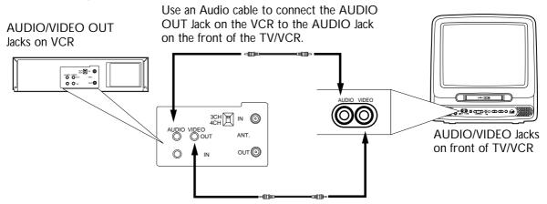
Use a Video cable to connect the VIDEO OUT Jack on the VCR to the VIDEO Jack on the front of the TV/VCR.
